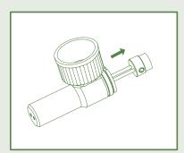
Slide out needle assembly from barrel.
