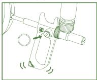
Loosen screw with coin. Adjust grip to adequate position. Lock screw.
