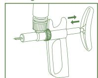
Activate handle a couple of times until liquid film is visible in needles.
