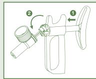
1 Activate handle and 2 slightly push barrel down to separate needles from handle.
