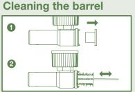
① Remove barrel cap. ② Clean inside with small brush and detergent solution. Rinse with water and dry.
