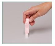
Dip the Reveal 3-D device into the liquid in the lid; ensure that the cavity is saturated with the liquid.
