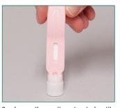
Leave the cavity saturated until the liquid is seen running into the test window.
