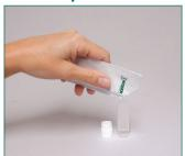
Open Type 3 extraction buffer sachet and add to a sample tube.
