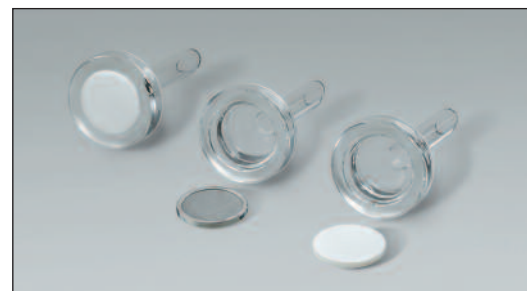
Glass frit, stainless steel support, PTFE support
