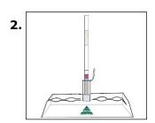
Take one AgraStrip® Cashew/Pistachio test strip from its container and place it vertically (sample pad downwards) into the incubation vial. Incubate for **5 minutes**.
