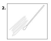
Wipe an area of **5 cm x 5 cm** using side-to-side movements, rotating the swab tip as you go. We recommend the "cross-hatch" swabbing technique indicated below.
