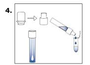
After shaking, remove the cap from the extraction tube and replace it with a dropper tip. Transfer **12 drops** or **400 \muL** into an incubation vial and close the lid.
