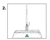
Take one AgraStrip<sup>®</sup> Crustacea test strip from its container and place it vertically (sample pad downwards) into the incubation vial. Incubate for **5 minutes**.
