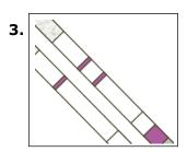
Remove the test strip directly after the 5-minute incubation period and read the result immediately.
