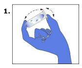
Shake the incubation vial vigorously by hand for **15 seconds**, making sure that the liquid comes in contact with the lid of the vial. Place the vial on the vial rack and let it rest at room temperature for **5 minutes**.
