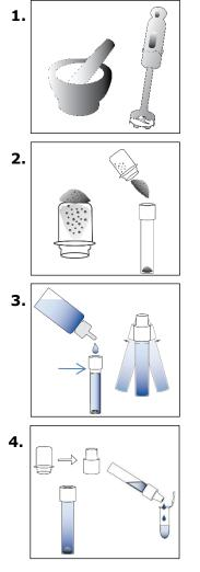
Obtain a representative sample of the specimen you want to analyze and homogenize it using a blender or a mortar and pestle. For rinse water samples, proceed to step 2.
