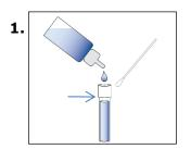
Fill one extraction tube with **extraction buffer** up to the bottom of the neck of the tube, as indicated by the arrow. Take a swab and wet its sampling end by dipping it into the buffer.
