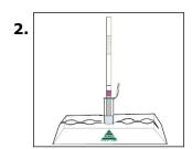
Take one AgraStrip<sup>®</sup> Gluten test strip from its container and place it vertically (sample pad downwards) into the incubation vial. Incubate for **5 minutes**.
