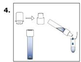
After shaking, remove the cap from the extraction tube and replace it with a fresh dropper tip. Then, transfer **12 drops** or **400 \muL** to an incubation vial and close the lid.
