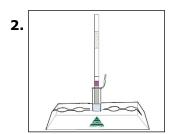
Take one AgraStrip® Hazelnut test strip from its container and place it vertically (sample pad downwards) into the incubation vial. Incubate for **5 minutes**.
