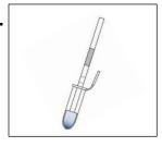
Insert a test strip into the solution and incubate at room temperature for **5 minutes**. **Read the result immediately**.
