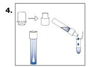
After shaking, remove the cap from the extraction tube and replace it with a dropper tip. Transfer **12 drops** or **400 \muL** into an incubation vial and close the lid.
