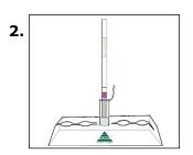
Take one AgraStrip<sup>®</sup> Lupin test strip from its container and place it vertically (sample pad downwards) into the incubation vial. Incubate for **5 minutes**.
